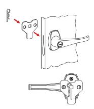
3. With the handle still in the open position, hook the locking bars (Ref. No. 13) to the locking cam (see "A" at left). Once in position, slowly rotate the door handle to the closed position so the lock bars prot rude from the holes at the top and bottom of the door (shown at right, below).
