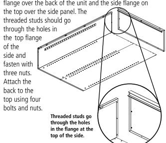
**5.** Attach the right side (Ref. No. 3) to the back in the same manner as you did in step 3, again, making sure that the flange is around the back and that the lances on the shelf adjustment strips are pointed in the same direction as those on the back and left side. Push the side panel up so the studs in the top go
